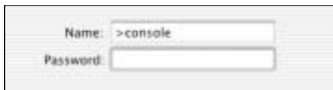
Figure 2.2 You can use the name “>console” to log in to the command line instead of Aqua.
